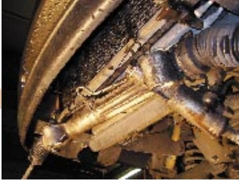
10.Remove brake calipers left & right
