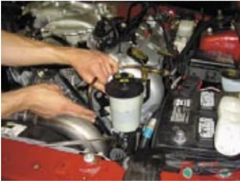
64. Hang down pipe to exhaust housing using supplied V-band clamp. Leave clamp loose. (Heat shield not shown with pic)
