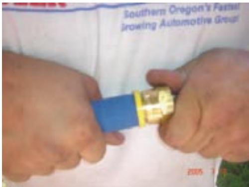
122. Install and tighten oil lines, \*note inlet and outlet\*
