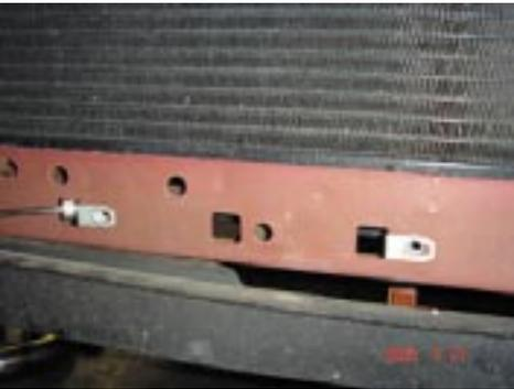
92. Install intercooler with supplied metric bolts. Bolt it to lower radiator support, leaving bolts loose.
