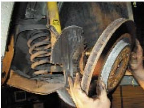
12.Remove ABS sensor lines both left and right
