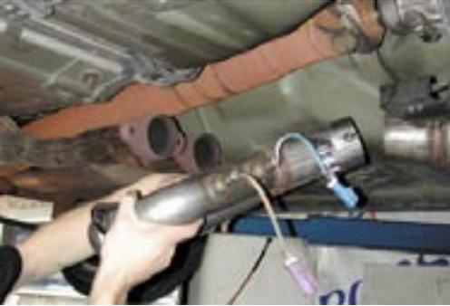
75. Bolt Y-pipe to mufflers.
