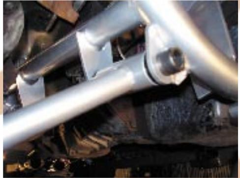
27. Install motor mounts nuts and tighten to 110 ft. lbs.
