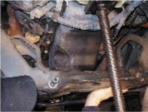
19. Support K-member and remove K-member bolts (6) attaching K-member to frame.
