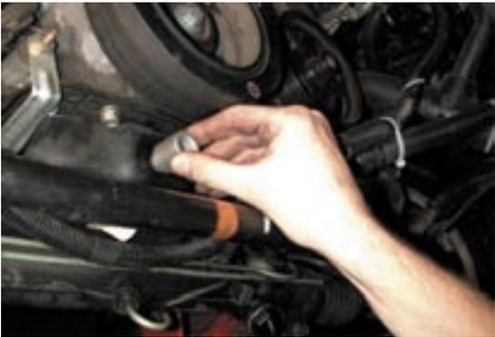
58. Next, take a 3/8" pipe tap (supplied) and coat it with grease. Tap hole in pan. The grease will catch the tapped shavings.
