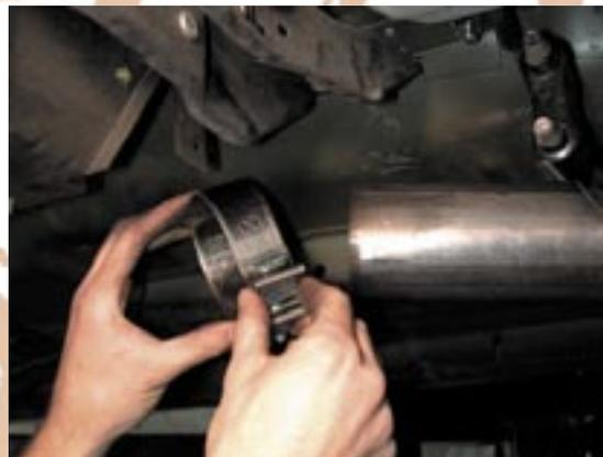
73. Install straight pipe or catalytic converter onto the "double barrel". Again, slide clamp on first.
