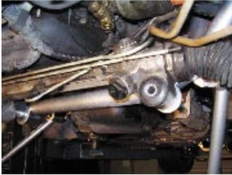
30. Re-install steering knuckle and tighten
