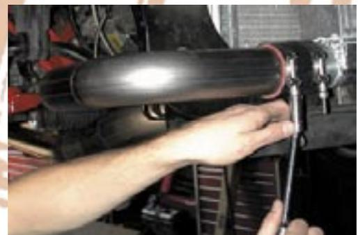
97. Install intercooler pipe #2 onto upper intercooler outlet.
