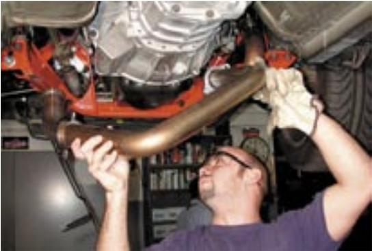
69. Bolt exhaust hanger to driver side transmission mount using supplied 5/16" bolt, nut and washer. This is the sheet metal bracket that is attached to the floor of the car.
