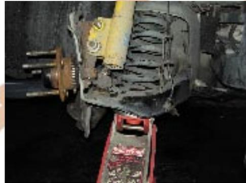
16.Remove spindle, both left and right
