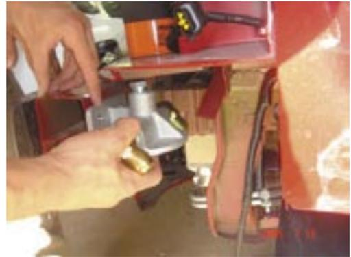
118. Drill bumper with 5/16 drill bit. The bumper is hardened steel, so multiple drill bits may be needed to reach the size required.
