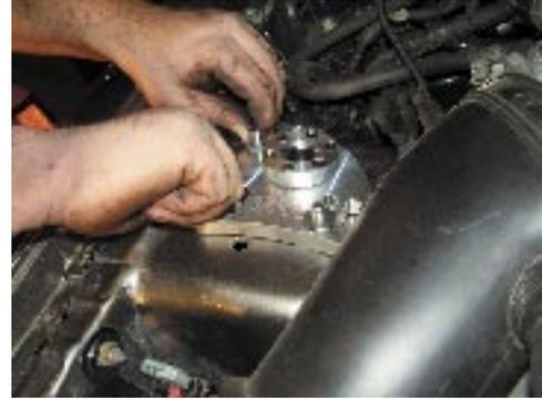
34. Install strut with coilover kit into caster/camber plate, using caster/camber instructions as reference for bearing/shim stacking order.
