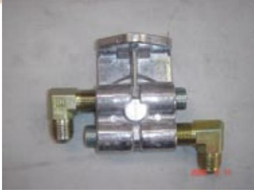
116. Install adapter onto engine and tighten
