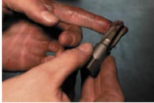
59. Remove tap and wipe the remaining grease from hole, being careful not to let shavings fall into pan.
