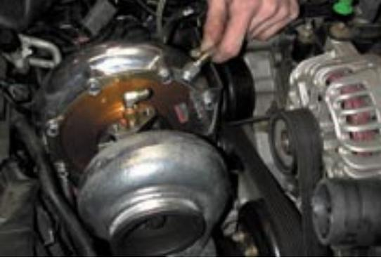
82. Install turbo oil outlet extension with pipe paste and tighten.
