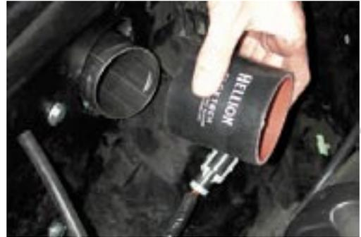
99. Install intercooler pipe #3 and silicone hose.
