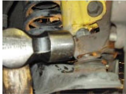
15.Support A-arm with jack to take load off of spring and remove the 2 strut to spindle bolts, then lower A-arm, being cautious because spring is under pressure.
