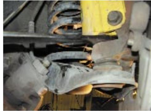
14.Use an air hammer or electric hammer with a pickle fork in order to disengage ball joint from spindle
