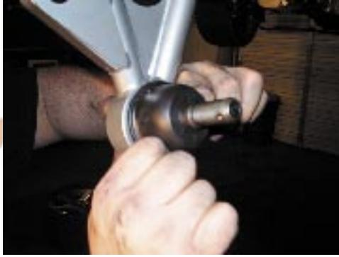
29. Install steering rack, install rack bolts and tighten
