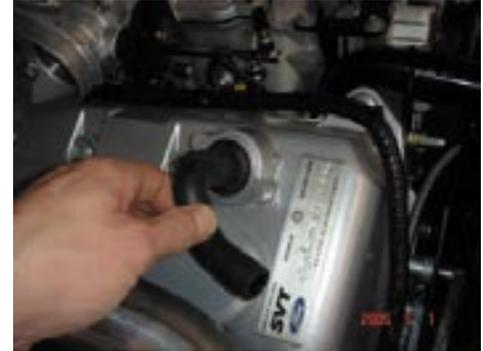
106. Attach the supplied vacuum line from the turbo compressor to the underside of the wastegate.
