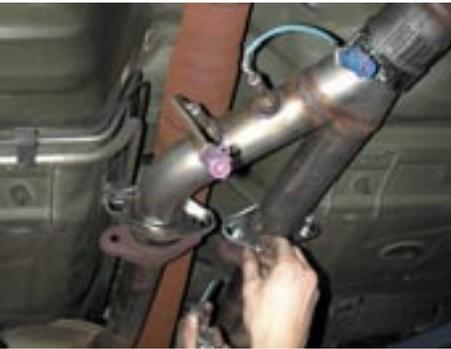
76. Position the entire exhaust system with about 1/2" clearance from other parts.
