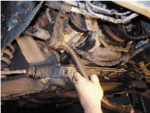
4. Remove steering shaft bolt
