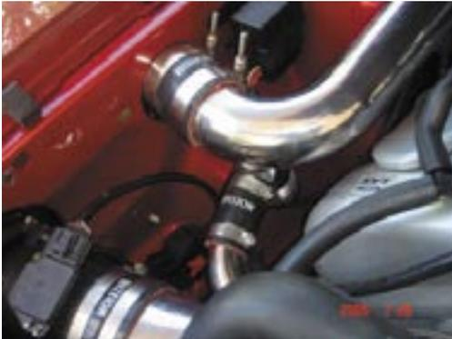
104. Position all intercooler pipes and tighten all clamps.
